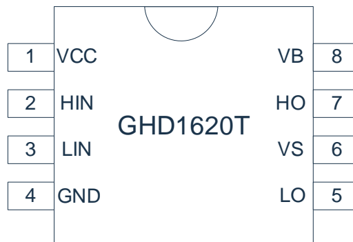
Figure 1 Distribution Diagram of GHD1620T Pins
